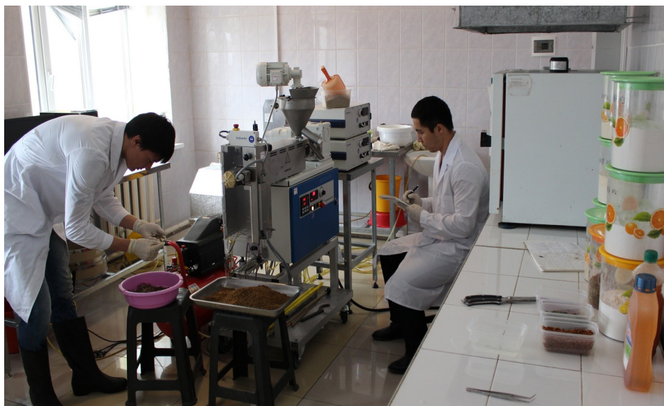
Figure 22 – The preparation of product feed by extruding method.
