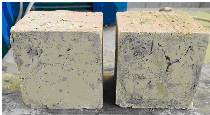
Picture 2 – Ground concrete with the addition of 20% cement
