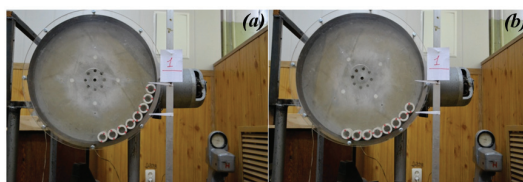
FIGURE 1. Motion of rods in the cross section of the rotating drum.
