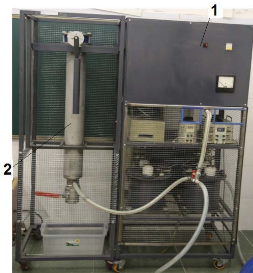
Figure 3. Ion-ozone cavitation installation: 1 – ion-ozone generator; 2 – cavitation capacity
