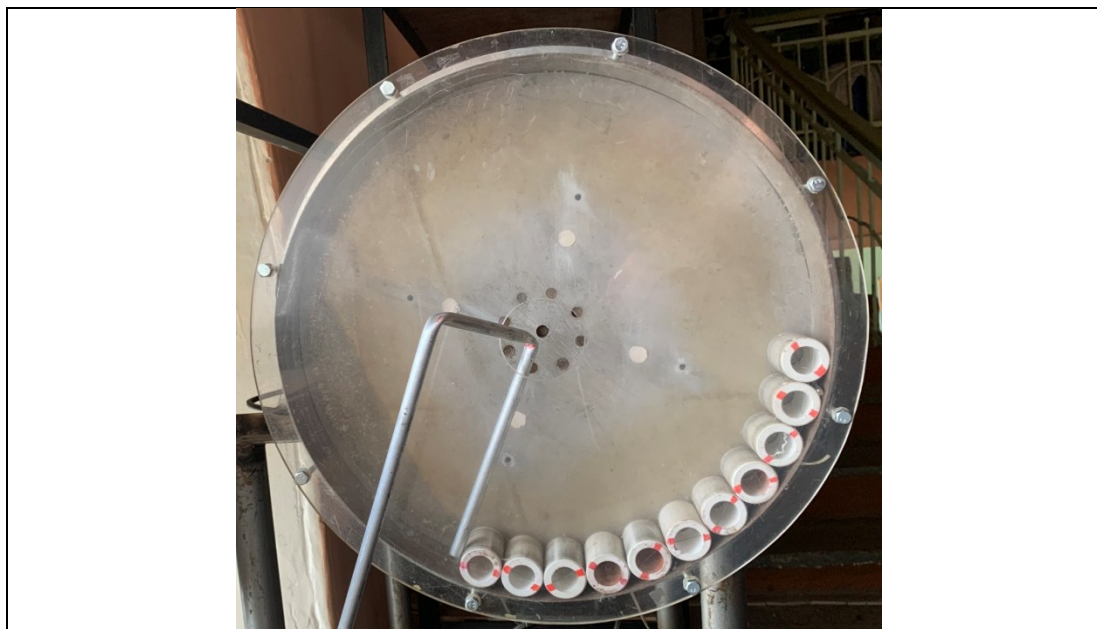
Figure 1. Rods connected by a flexible cable in a rotating drum.
