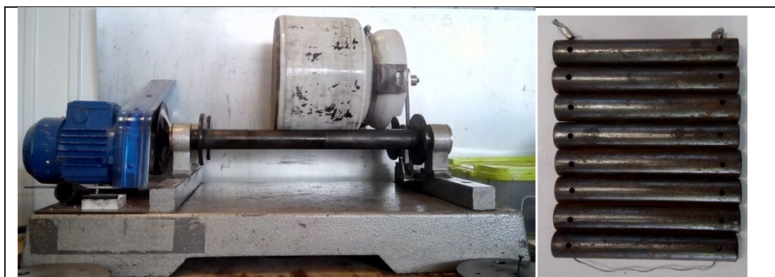
Figure 2. Laboratory ball mill (a) and grinding rods (b).
